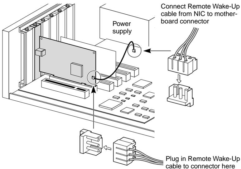
**Figure 2-3** Connecting the NIC to the Connector
