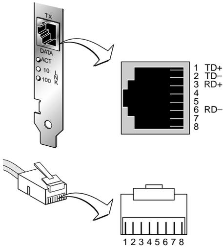
**Figure A-1** RJ-45 Connector Pin Assignments
