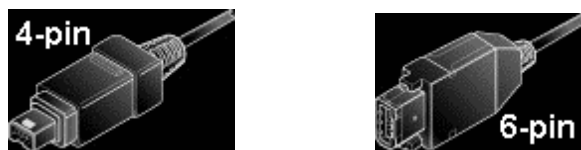
Picture 4: 4-pin and 6-pin FireWire connectors
