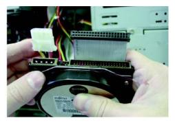
**4** Attach the power connector to the new hard disk. There is only one way to connect the power cable-do not force it. Make sure the angled edge of the plastic connector lines up with the angled edge of the pin socket.
