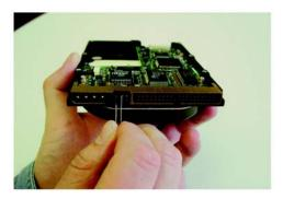
**3** Attach the new hard disk. Connect the cable so that the colored stripe on the edge lines up with the I/O pins on the motherboard. The motherboard is marked Pin1 or 1 where the colored stripe should go. Next, connect the other end of the cable to the back of the hard disk, again matching the striped edge with the I/
